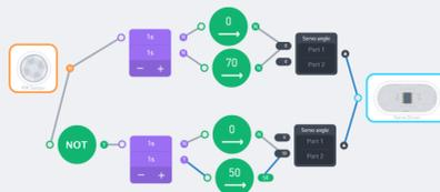
Example: when there is a person in front of the device (detected by the PIR sensor), nod head by repeatedly shaking the servo attached to port 1; otherwise, shake head by repeatedly shaking the servo attached to port 2.
