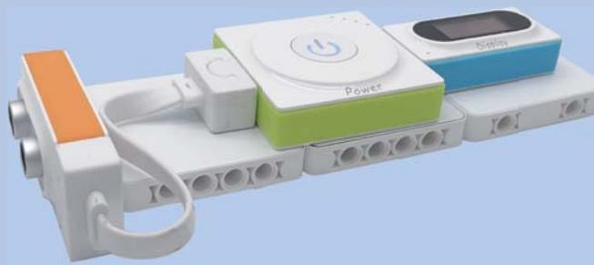
**Example Details:** Measure the distance from the ultrasonic sensor to an obstacle. Use the display block to show the value.
