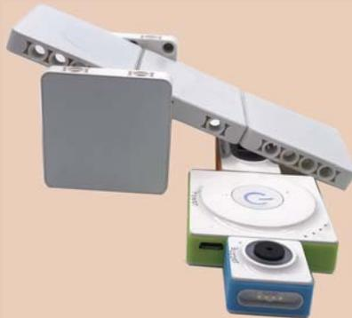
**Example Details:** The example is called Morse Telegraph. Tap the magnetic plate rhythmically and the buzzer will make sounds according to the rhythm. Try sending a group of encoded messages for seeking help?
