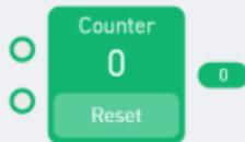
When the input changes from “no” to “yes”(we call it a “rising edge” in electric engineering), the number displayed in the node will plus one, and goes to the output. If you push the “reset” button, the number will be reset to zero; the same will happen if the “RESET” input changes from “no” to “yes”.
