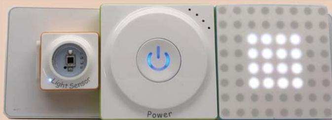
Example Details: The light sensor detects the light intensity of environments. The brightness and number of lights on the LED panel vary according to signals from the input block. (When the light intensity is strong, the LED lights will be brighter and the number of lights will be larger; otherwise, the lights will be darker and the number will be smaller. )
