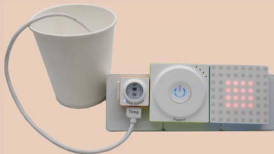
**Example Details:** The temperature value of the the water determines the brightness of the LED panel( expansion).
