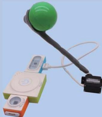
**Example Details:** Design a catapult. Change the rotation angles by controlling how the gyro sensor vibrates.
