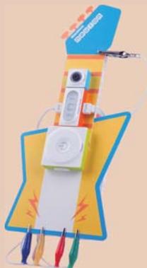
**Example Details:** Take turns touching alligator clips of different colors and touch the GND wire clip with the right hand. Listen, the buzzer is making different sounds.
