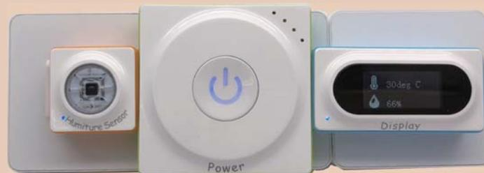
**Example Details:** After the sensor finishing detecting the temperature and humidity of an environment, the LED display will show the value.
