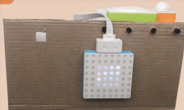
**Example Details:** Make a lighting panel. The larger the knob value is, the brighter the LED panel will be.
