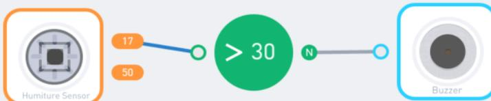
When the temperature is over 30 (degrees Celsius), sound the buzzer.
