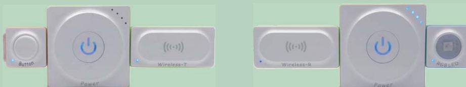
**Example Details:** Pair the wireless transmitter block and the wireless receiver block. Then connect the wireless transmitter block to the input block and the wireless receiver block to the output block; the input block can remotely control the output block.
